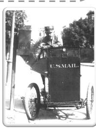
Photo from 1912 shows a motorized cart that was designed to receive mail from the boxes via a chute that dumped directly into the cart.
